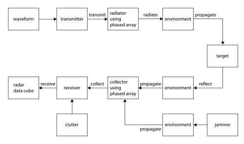
To exploit the advantages of array processing, you must first understand how to model and optimize the performance of each component and operation in a phased array system. This software provides models for all the components of the phased array system illustrated in the preceding figure from signal synthesis to signal analysis.
